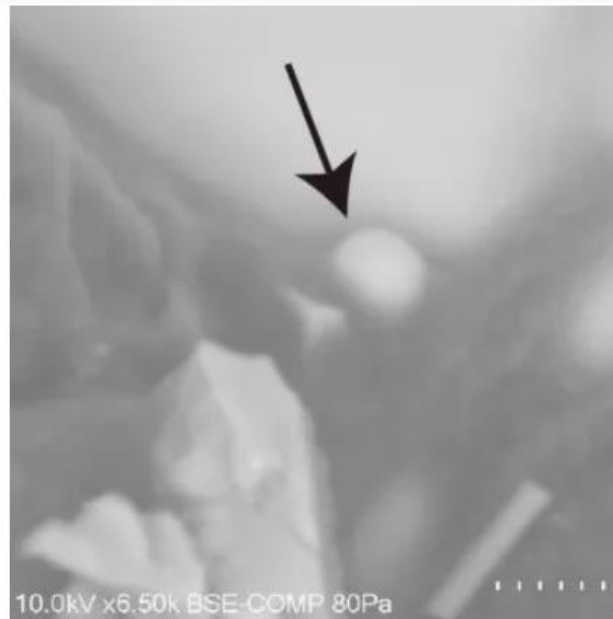
The first electron microscope view of the previously unknown radioactive cesium microparticle, from air filter samples collected in Tsukuba, about 100 miles from the Fukushima nuclear plant. (Adachi et al. 2013)
